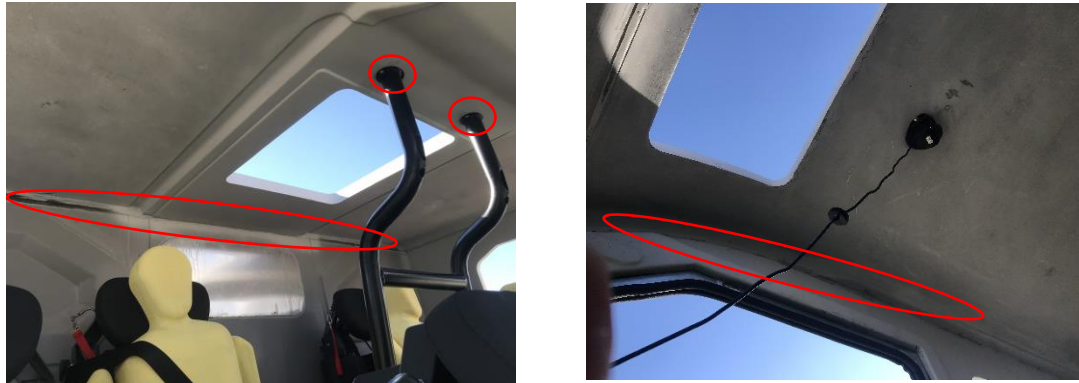
Figure 12. Roof Strength Test 2 of Failure Assessment (Test C2)
