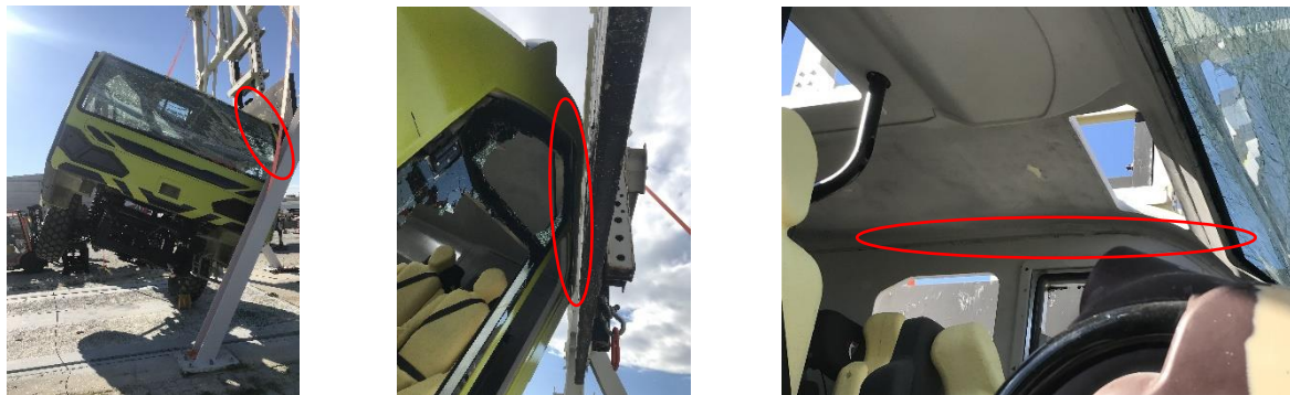
Figure 11: Roof Strength Test 1 of Failure Assessment (Test C1)
