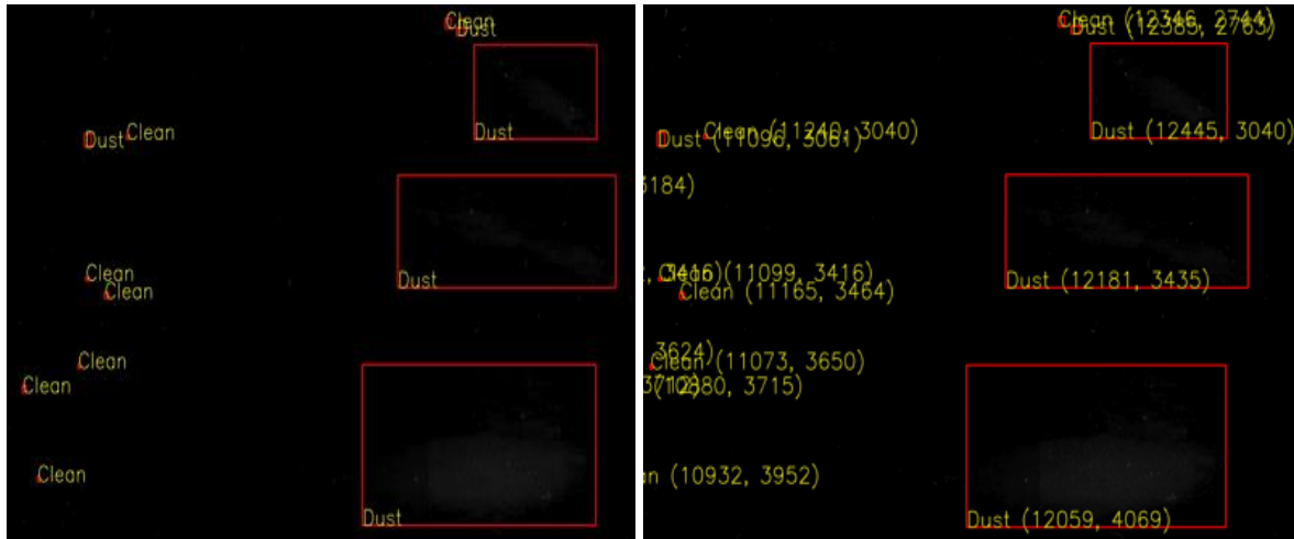
Figure 14: The location, size and names of the defects are plotted in pixels on the acquired glass image.
