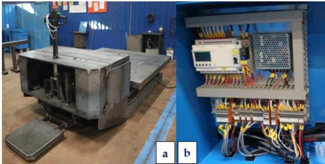
Figure 1: a. Mechanical Parts, b. Automation System of Produced Prototype
