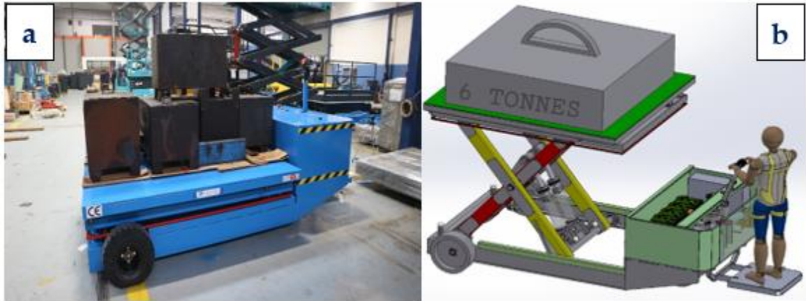
Figure 2: a. Prototype Image, b. Operator Stand Model of Mobile Scissor Lift Platform
