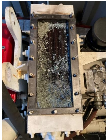
Figure 2: Fouling in Fin-and-Tube Heat Exchanger
