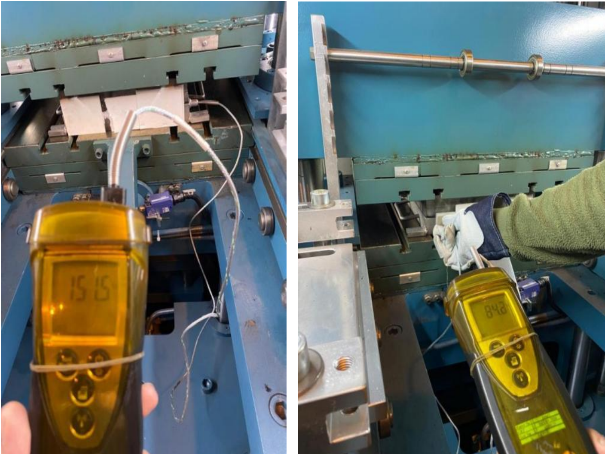
Figure 1. Non-insulated outer surface temperature and outer surface temperature of mounted ceramic plate
